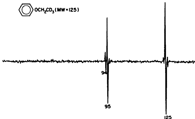
Fig 1. ICR spectrum of phenyl 2,2,2-trideuteroethyl ether, \omega_1/2\pi = 153.6 kHz, 2 \times 10^{-6} Torr, 20 eV. Further instrumental conditions relevant to this and following figures are described in the experimental part.
